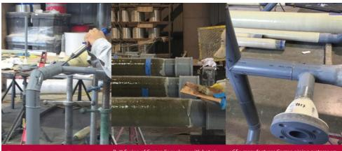
Thorpe adheres to strict in-house QA/ QC practice. This is vital for application reliability. Butt Fusion of Corzan liner along with hot air gas welding gives you the ability to produce complex fabricated systems
